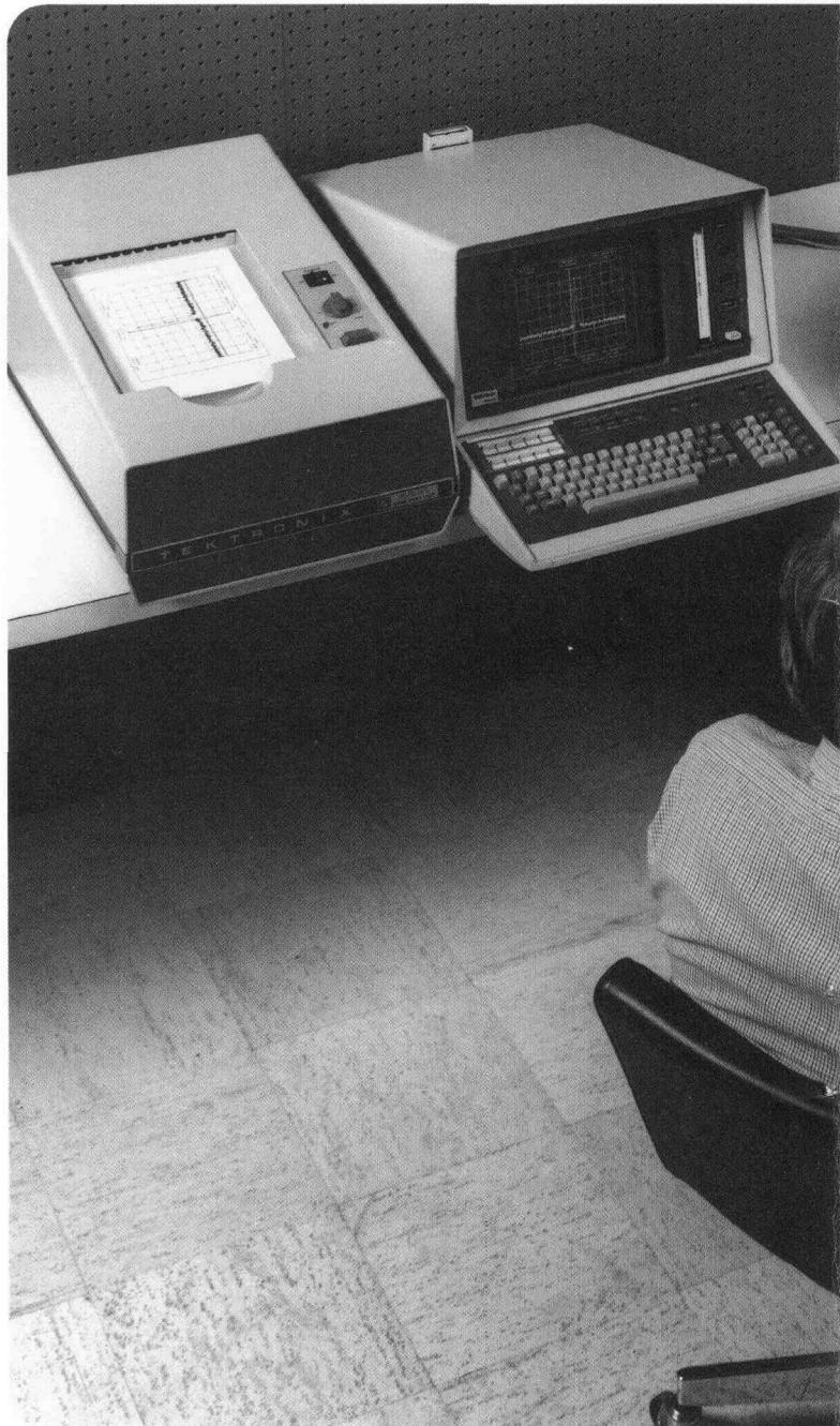
When used with the Tektronix 4052 Graphic Computing System controller and 4631 Hard Copy Unit, the 492P can provide test results in both graphic and numeric form for the evaluation of microwave signal sources.
